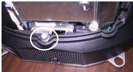
FIGURE 35 - SCREW IN CENTER OF BOTTOM COVER
