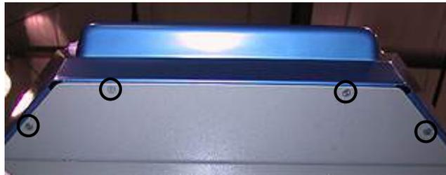
FIGURE 22 - FRONT OF SHROUD FASTENED WITH SCREWS
