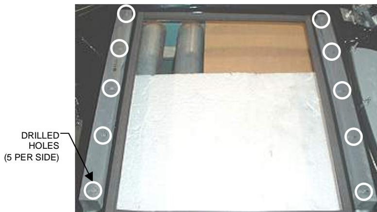
FIGURE 15 - FORCE FUSION - PLASTIC MOUNTING PIECES ON BEZEL
