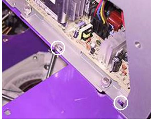
FIGURE 27 - POSSIBLE HARDWARE LOCATION FOR MOUNTING MONITOR
