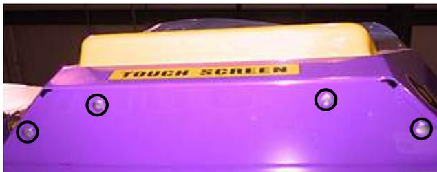
FIGURE 23 - FRONT OF SHROUD FASTENED WITH BOLTS
