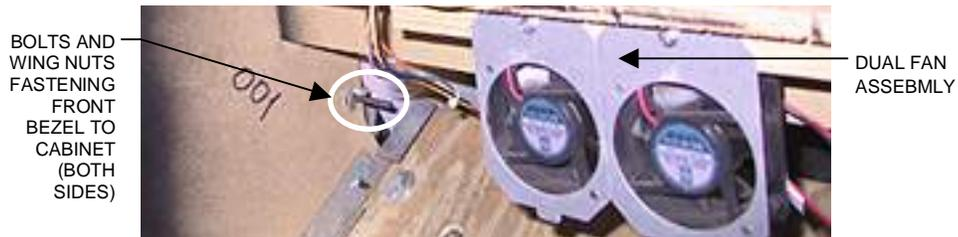
BOLTS AND WING NUTS FASTENING FRONT BEZEL TO CABINET (BOTH SIDES)
