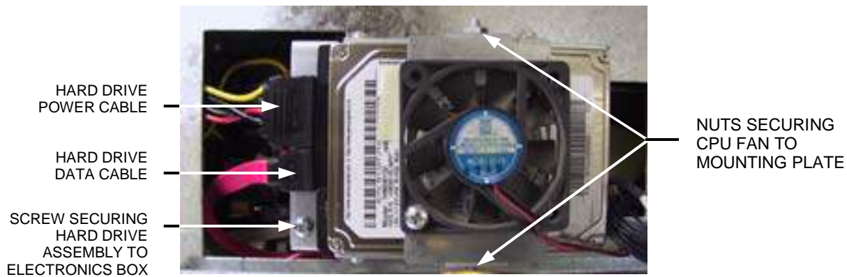
FIGURE 6 - SATA HARD DRIVE ASSEMBLY ON ELECTRONICS BOX
