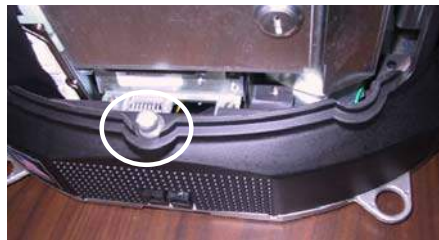
FIGURE 2 - SCREW IN CENTER OF BOTTOM COVER
