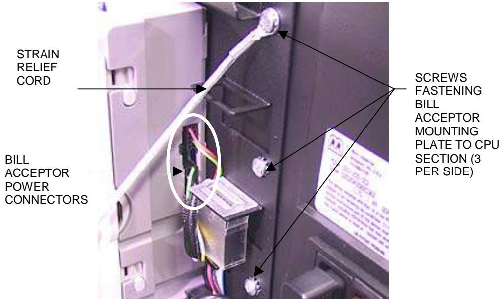
FIGURE 2 - REAR VIEW OF BILL ACCEPTOR MOUNTING PLATE
