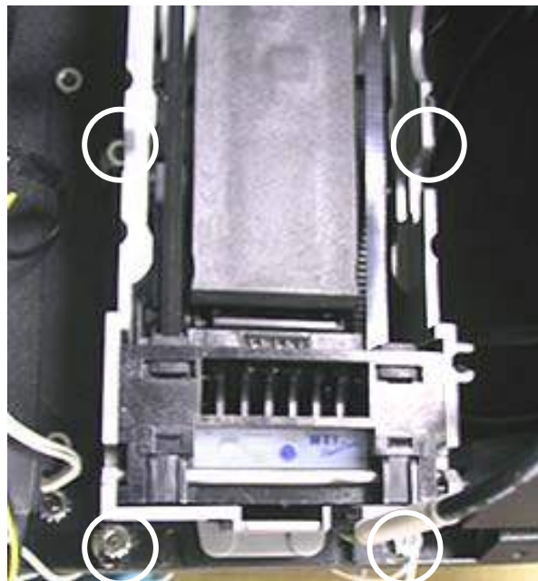
FIGURE 4 - SCREWS SECURING BILLACCEPTOR TO MOUNTING PLATE
