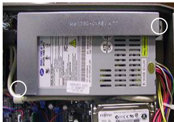
FIGURE 2 - POWER SUPPLY MOUNTING SCREWS (2 PLACES)
