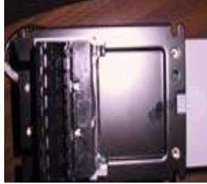
FIGURE 11 - METAL MOUNTING PLATE UNDERNEATH BILL ACCEPTOR BEZEL
