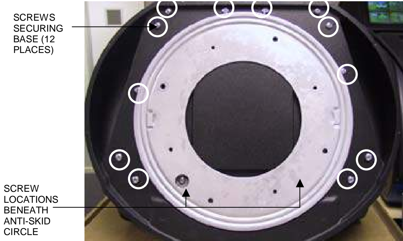
FIGURE 2 - ELITE EDGE - BASE AND ANTI-SKID CIRCLE REMOVAL
