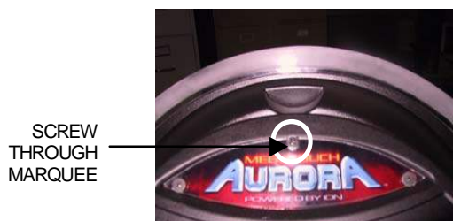
FIGURE 3 - SCREWS ON FRONT AND BACK OF BEZEL
