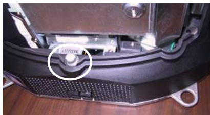
FIGURE 2 - SCREW IN CENTER OF BOTTOM COVER
