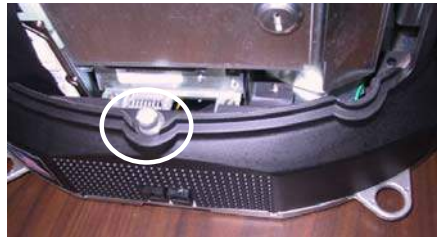
FIGURE 2 - SCREW IN CENTER OF BOTTOM COVER
