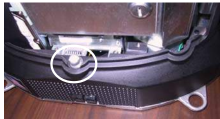
FIGURE 2 - SCREW IN CENTER OF BOTTOM COVER
