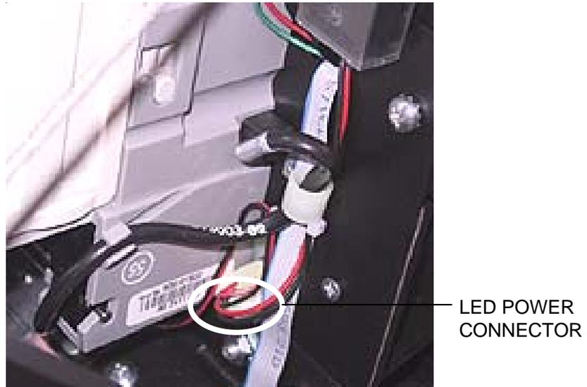
FIGURE 9 - REAR VIEW OF CPU SECTION
