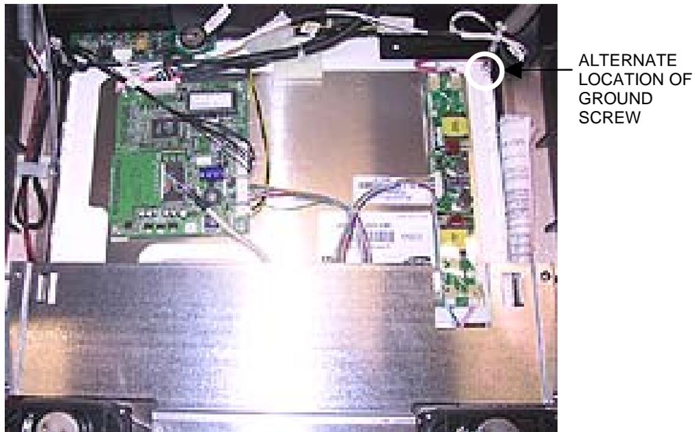
FIGURE 8 - CLOSEUP OF CPU SECTION, LCD MONITOR WITH EXTERIOR CIRCUIT BOARDS
