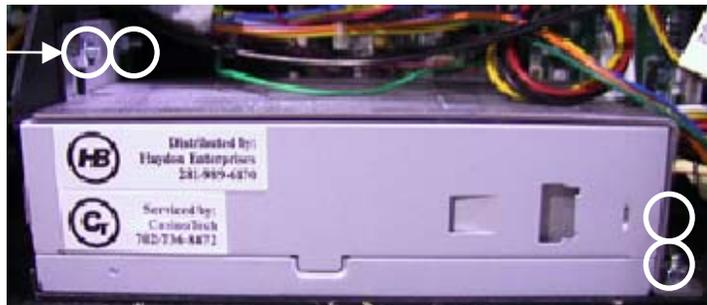
FIGURE 5 - POWER SUPPLY AND MOUNTING BRACKET
