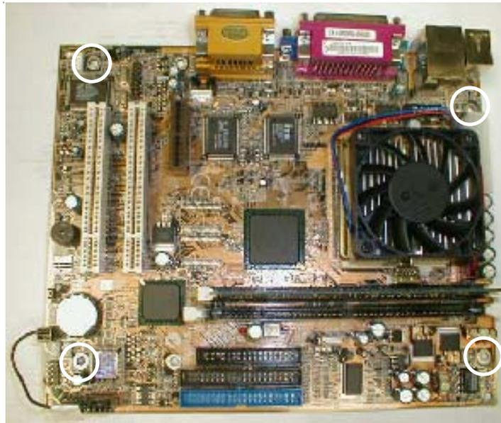
FIGURE 1 – MOTHERBOARD REMOVAL –
