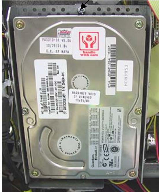
FIGURE 1 – HARD DRIVE REMOVAL
