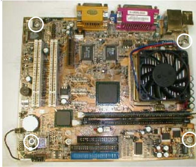
FIGURE 1 – MOTHERBOARD REMOVAL –
