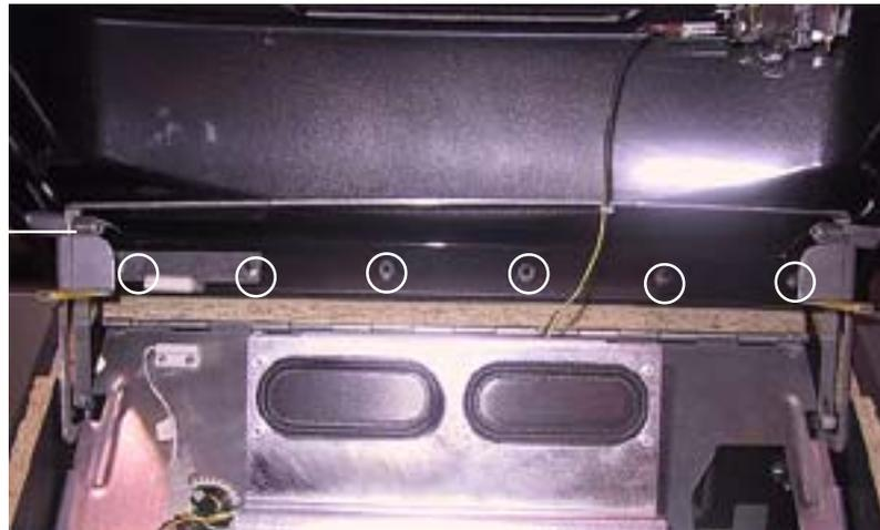
FIGURE 10 - SCREWS AND HEXNUTS SECURING HINGE - UNDER TOP BEZEL
