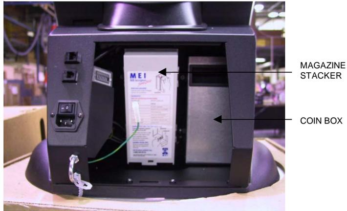
FIGURE 19 - ELITE EDGE - BILL ACCEPTOR ACCESS/REMOVAL
