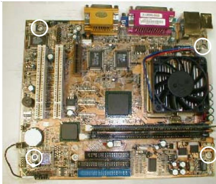
**FIGURE 2 - MOTHERBOARD REMOVAL -
