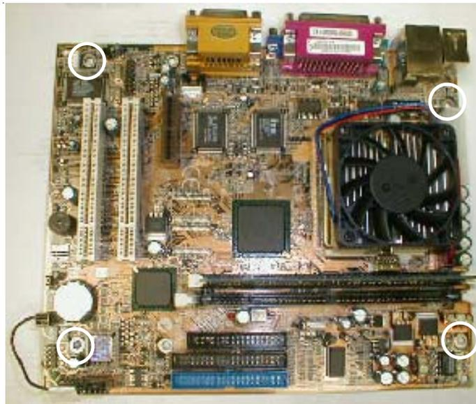
FIGURE 2 – MOTHERBOARD REMOVAL –
