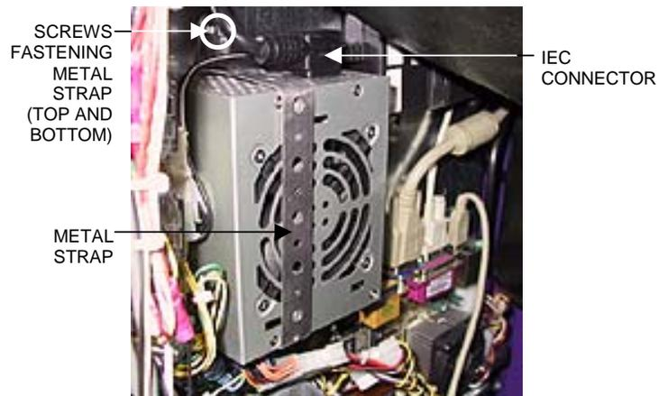
FIGURE 5 - CLOSEUP OF POWER SUPPLY WITH METAL STRAP
