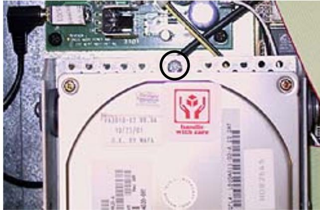
FIGURE 2 - HARD DRIVE REMOVAL -
