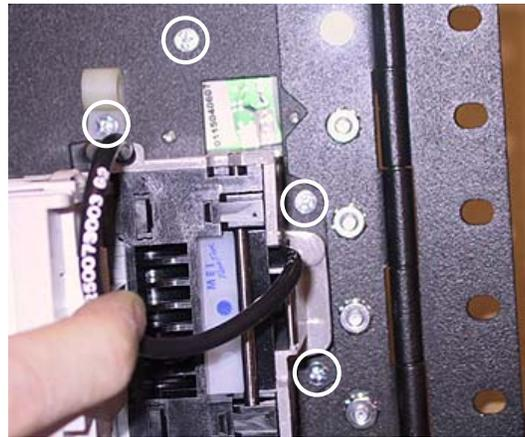
FIGURE 17 - SCREWS FASTENING BILL ACCEPTOR BEZEL TO MOUNTING PLATE
