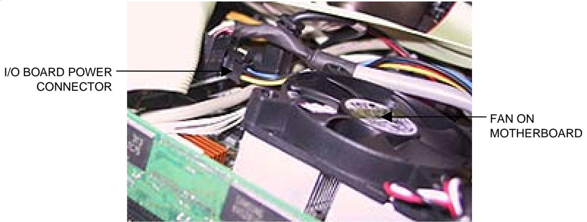
FIGURE 11 - CLOSEUP OF MOTHERBOARD
