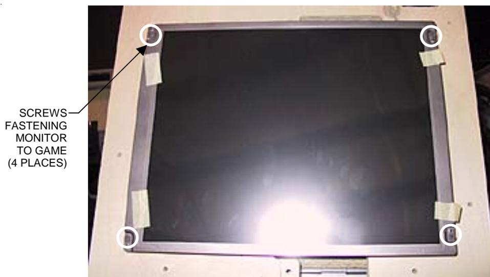
FIGURE 5 - MONITOR (WITH BEZEL REMOVED)
