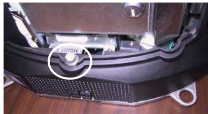
FIGURE 2 - SCREW IN CENTER OF BOTTOM COVER
